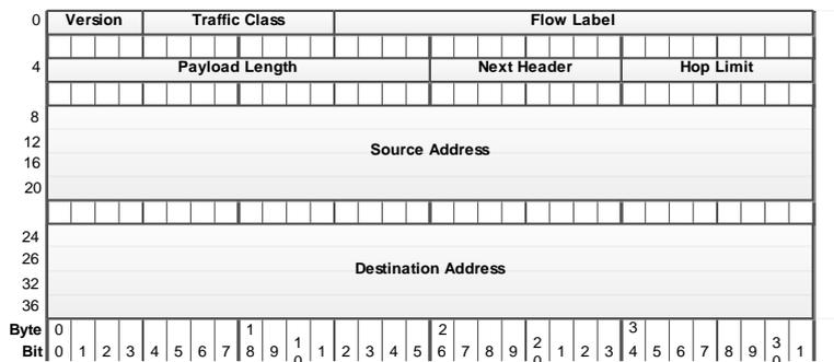
The IPv6 header structure
